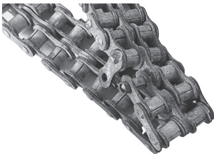
Corrosion of stainless steel drive chain
